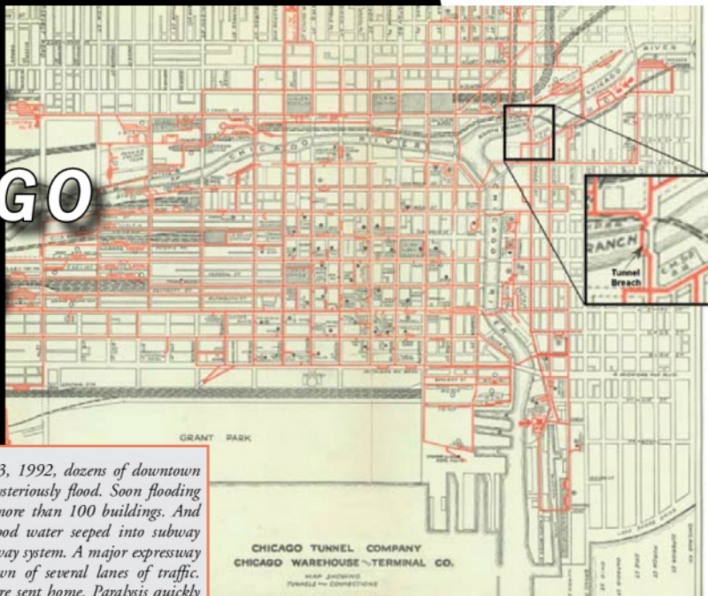
Figure 1: Chicago freight tunnel network and location of tunnel breach beneath the North Branch of the Chicago River at the Kinzie Street crossing. (Source: What the Freight Tunnels Mean to Chicago , Chicago Freight Tunnel System, Chicago Tunnel Terminal Corporation, 1928.)
