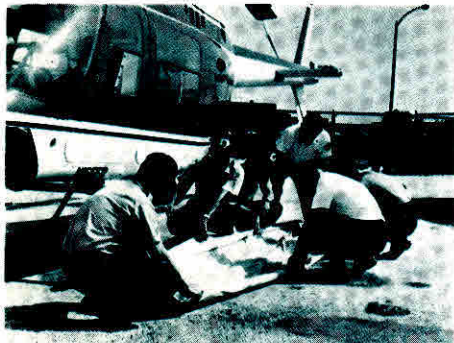
Lt. George Tannehill (at rear) supervises the packing of stowed floats on JetRanger. In-flight inflation takes 3½ seconds for over water operations.
